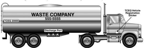
Figure 1. Example of vehicle marking and sticker placement.
